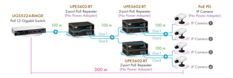
\*\* Note: If the Ethernet cable is not standard CAT5 cable, the UPE5600-RT may be working for shorter length than 100 meter.
