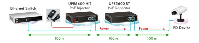
\*\* Note:If the Ethernet cable is not standard CAT5 cable, the UPE5600-RT may be working for shorter length than 100 meter.
