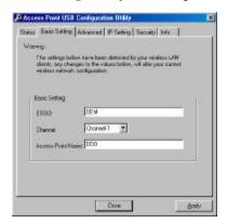
**ESSID:** ESS stands for "Extended Service Set". The ESS ID is the name shared among all points in a wireless network system. The ESSID must be identical for all points in the system and must not exceed over 30 characters. After changing, please click "Apply" button for setup. Default will be "OEM".
