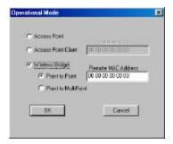
Wireless Bridge: This mode allows the connection of one or more remote LANs with a central LAN, creating thus an extended single virtual LAN. In this way, any station of the Remote LAN can successfully communicate with any station of the central LAN, as if all of them belonged to the same physical LAN. Wireless station can't associate with wireless bridges. The Access Point conducts the designated traffic to the appropriate wired or wireless station.
