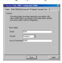
**ESSID:** ESS stands for "Extended Service Set". The ESS ID is the name shared among all points in a wireless network system. The ESSID must be identical for all points in the system and must not exceed over 30 characters. After changing, please click "Apply" button for setup.
