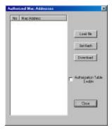
The **Load file** button is to load a file with the MAC Addresses that can be associated with the Access Point. The user can type in the MAC Addresses which are permitted to access into this WLAN network.
