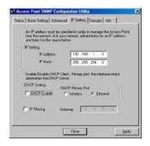
IP Address: The IP address of Wireless Network should be different as the network IP addresses.
