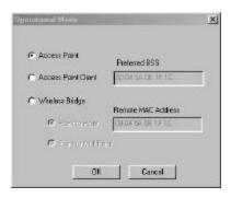
**Access Point:** This mode provides access for wireless stations to wired LANs and from wired LANs to wireless stations. Furthermore, wireless station within the range of the Access Point device may communicate with each other via the Access Point. In this option the Access Point is as a base station to build up a basic Wireless Local Area Networking.
