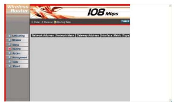
**Network Address:** Displays the network IP address of the connected node. **Network Mask:** Displays the network (subnet) mask of the connected node.
