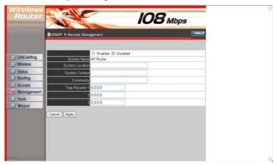
**Enabled/Disabled:** Click to enable or disable SNMP. **System Name:** Displays the name given to the router.
