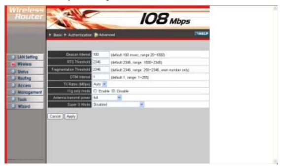
**Beacon Interval:** Type the beacon interval in the text box. You can specify a value from 1 to 1000. The default beacon interval is 100.
