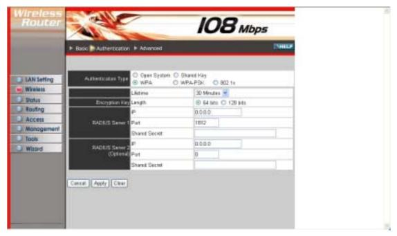
**Lifetime**: Select the Lifetime of the Encryption Key from 5 Minutes to 1 Day. As soon as the lifetime of the Encryption Key is over, the Encryption Key will be renewed by the Radius server.
