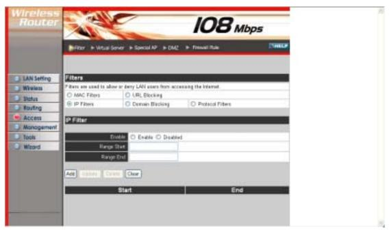
**Enable:** Click to enable or disable the IP address filter.
