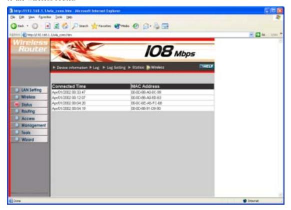
**Connected Time:** Displays how long the wireless device has been connected to the LAN via the router.
