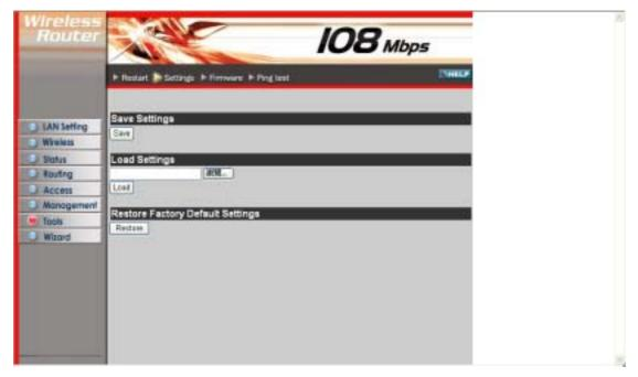
**Save Settings:** Click to save the current configuration as a profile that you can load when necessary.
