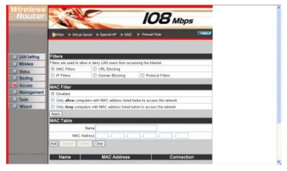
**MAC Filter:** Enables you to allow or deny Internet access to users within the LAN based upon the MAC address of their network interface. Click the radio button next to *Disabled* to disable the MAC filter.
