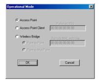
Access Point: This mode provides access for wireless stations to wired LANs and from wired LANs
