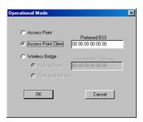
**Access Point Client:** In this option, the Access Point can be a base station in a WLAN system, but also as a client station to communicate with other stations in the WLAN system.
