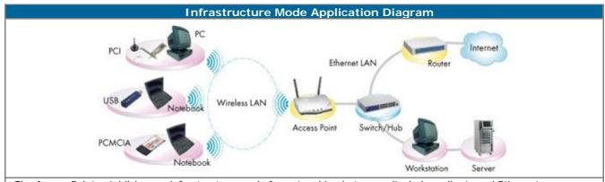
The Access Point establishes an infrastructure mode for networking between all wireless clients and Ethernet resources.
