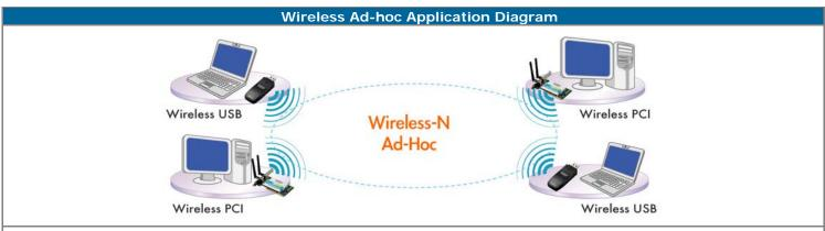
The wireless Ad-hoc mode is established by several wireless clients, which have the same SSID and radio channel. The wireless USB/PCI/PC Card adapters can be used for such peer-to-peer communication mode.
