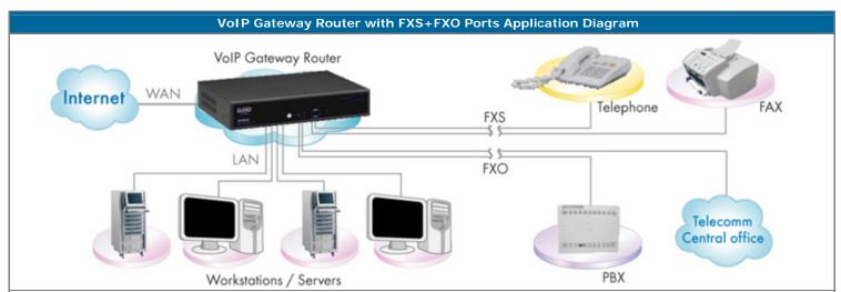
The VoIP Gateway with router making voice and data connectivity together with IP sharing router function. Telephone and fax can be served by FXS port and other FXO ports support telecom central office line or PBX.
