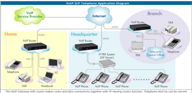
The VoIP Gateway with router makes voice and data connectivity together with IP sharing router function. Telephone and fax can be served by FXS port and other FXO ports support telecom central office line or PBX. The IP phone is a full-featured, cost-effective, and standard-compliant VoIP telephone that can be easily plugged to your home or office network with Ethernet cable.
