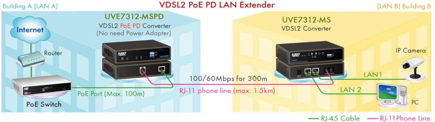
A pair of VDSL2 converters with PoE PD featured that takes power supply over Ethernet cable from PoE Switch is the best solution for bandwidth-hungry applications such as video streaming and FTTB over telephone line to extend connection for long distance.
