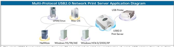
This single USB2.0 port print server allows any PC on a network to print any combination of variety USB printers through multiple operating systems and protocols support for maximum printer efficiency.
