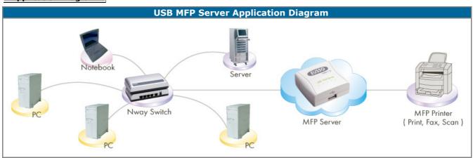
The MFP Server provides a 10/100Mbps LAN port for an easy way to share Print, Scan and Fax functions via latest generation of bi-directional USB multi-function printers.
