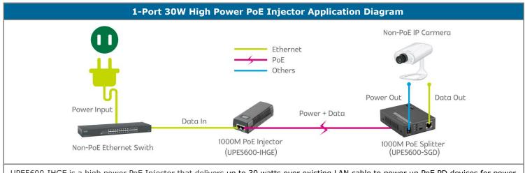
UPE5600-IHGE is a high power PoE Injector that delivers up to 30 watts over existing LAN cable to power up PoE PD devices for power hungry applications such as Wireless Access Points (AP), Security Cameras and IP Phones at farther distance.
